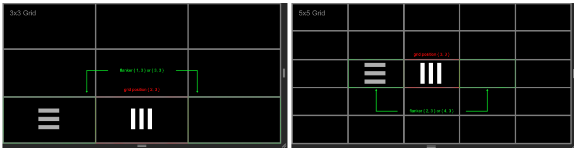
Fig. 3. Locations of two gratings stimuli from Mysore Lab's late-stage Shaping 8A visual paradigm are shown relative to a 3x3 and a 5x5 calibration grid on a 800x400 px screen. The text overlays shown were for labeling purposes only and are not present in the RAIL GUI.
